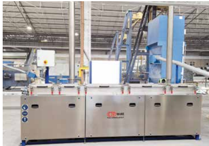
Nassbeschichtung NRB-3 / Wet coating machine NRB-3
