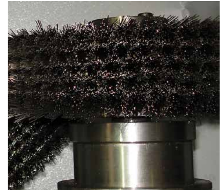
Detail Rundbürstanlage / Detail brush descaler
