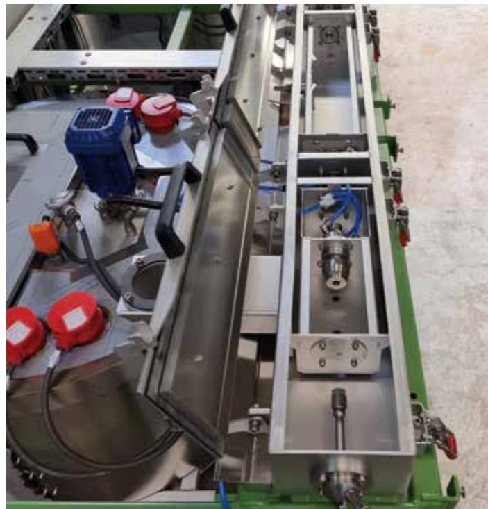
Nassbeschichtung NRB-3 / Wet coating machine NRB-3
